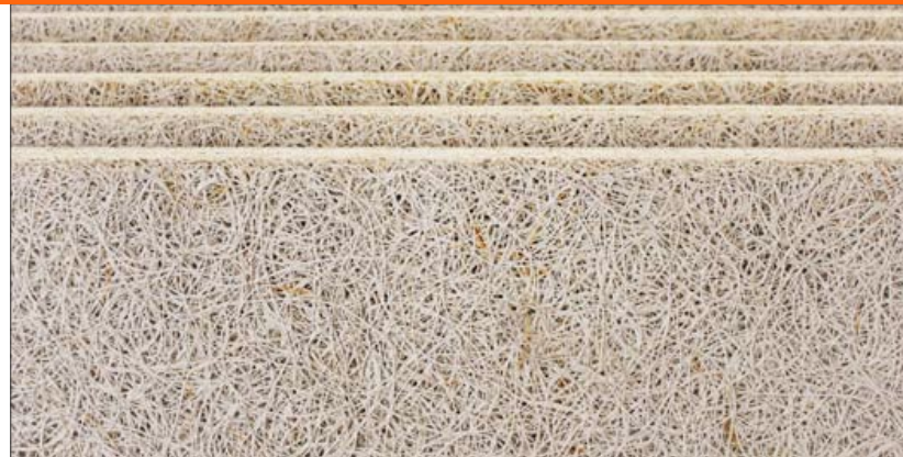
Sound-absorbing tectum panels await installation in the band and choral classrooms.
